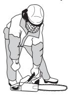
As the chain brake is still activated the engine must return to idling speed as soon as possible by disengaging the throttel latch in order to avoid unnecessery wear on the clutch assembly.
